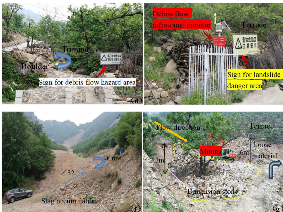
Figure 4. Huangsongyu National Mining Park. d is debris flow hazard area, e is debris flow monitoring instrument, f is loose slag accumulated in formation area and g is excavator mining.
